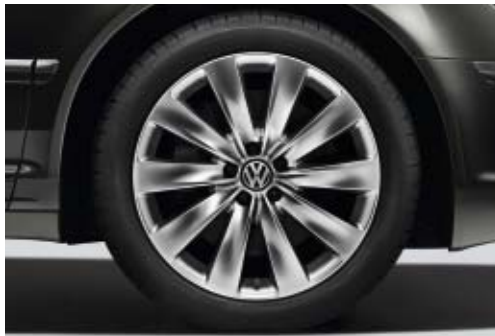
Four “Serres” alloy wheels, 8½ J x 19, 255/40 R 19 tyres. Painted Sterling Silver. With 245/45 R 19 tyres on W12.
