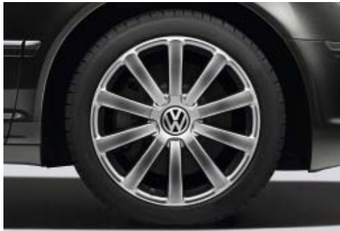
Four “Omanyt” alloy wheels, 9 J x 19, 255/40 R 19 tyres. Rims with bright finish.
