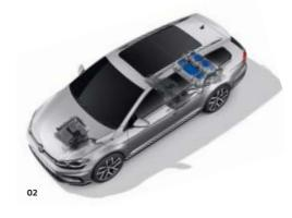
01|02 The natural gas drive reduces consumption and has a positive effect on emissions. The natural gas tanks are hidden underneath the floor to save space, so that they do not restrict the vehicle's flexibility or its storage space. And if the natural gas tank is empty, the additional petrol tank will easily take you to one of the 900 natural gas fuelling stations across Germany.
