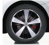
The **18 inch "Twister" alloy wheel**<sup>1)</sup> with size 235/45 R 18 tyre adds an extra portion of dynamics. |so
