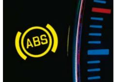
The anti-lock brake system (ABS) retains the steerability of the vehicle when full braking is applied, even on slippery surfaces. To give other road users due warning, the hazard warning system is activated at the same time.
