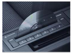
The CD changer in the front centre armrest helps you to put on audio CDs and can take up to six discs.
