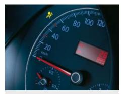
Blue illumination for the adjustable instrument cluster and instruments in the cockpit make them easy to read, independent of lighting conditions.
