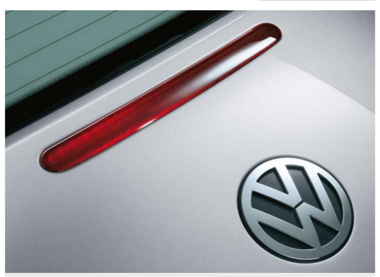
The **third brake light** with LED technology is neatly integrated in the rear lid and increases visibility on the road. It lights up in a flash when the vehicle is braked and therefore improves the reaction times of other road users.
