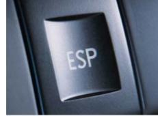
The electronic stabilisation programme (ESP) prevents the vehicle breaking away in critical situations through targeted intervention in the brake and engine management to assure maximum directional stability.
