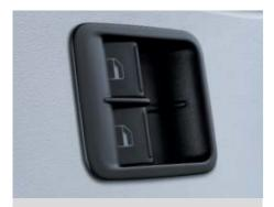
The electric windows in the De luxe package conveniently regulate the supply of fresh air. They have an important anti-trap feature for your safety: as soon as resistance is registered between the window and frame, the window is lowered a short distance.
