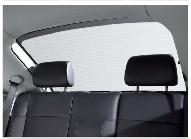
The **sun shade** for the rear window protects rear passengers from direct radiation from the sun without impairing the view to the rear and therefore road safety.
