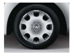
The 16 inch wheel package with 6  $\frac{1}{2}$  J x 16 wheels and 205/55 R 16 tyres also includes a set of full wheel trim.
