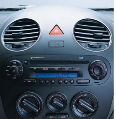
The MP3 compatible "gamma Volkswagen Sound" radio has eight loudspeakers, output of  $4 \times 20$  watts, a 30-station memory, and traffic information memory (TIM).
