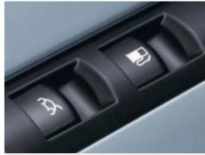
The remote control release for the fuel flap and luggage compartment opener are very practical features. This means that you do not have to get out of the vehicle to open the boot or fuel flap for others.
