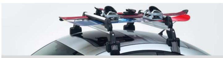
The lockable "comfort" ski and snowboard holder can carry up to six pairs of skis or four snowboards safely and conveniently. A practical pull-out function helps take the effort out of loading and unloading.
