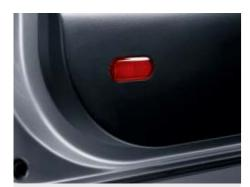
Door entry reflectors on the interior door panel trim are an additional safety factor in traffic as drivers of cars behind can immediately see when you open the door.
