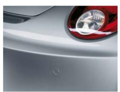
The ParkPilot has sensors in the rear bumper. During parking, acoustic and visual signals are given to warn of obstacles. The warning tone becomes more rapid as obstacles are approached.
