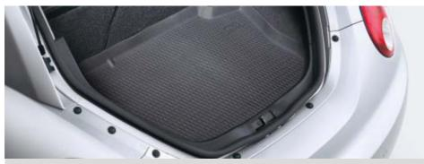
The **luggage compartment liner** has a close fit, is flexible and non-slip. It protects the luggage compartment of your New Beetle and can be wiped clean. The transparent **loading edge protective film** fits exactly to protect the rear bumper when loading and unloading.
