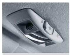
The Technical package includes an anti-theft warning system with interior monitoring. With the help of sensors, the system reacts if there is any manipulation on the bonnet, doors or rear lid.
