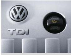
Direct diesel injection assures high pulling power for the **TDI engines** and, at the same time, low consumption coupled with minimal emissions. The exhaust turbocharger makes high engine output possible, even with small cubic capacity.
