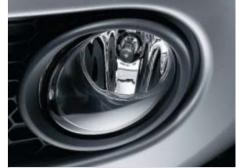
Fog lights belong to the Winter package. They improve illumination of the road in conditions of poor visibility and are therefore to be recommended as part of the safety equipment.
