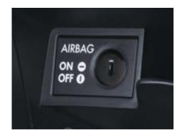
The **front passenger's airbag can** of course **be deactivated** – this is particularly important if you want to instal a child's seat on the front passenger side.
