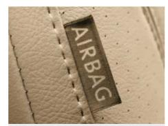
The combined head and side airbag system for the driver and front passenger is housed in the sides of the front seats. The airbags are triggered within a few milliseconds in the event of a collision and are filled by a gas generator.
