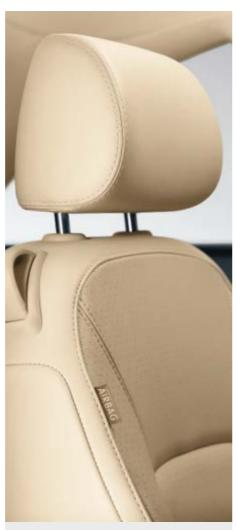
The safety-optimised head restraints are height-adjustable and minimise the risk of strain on the neck muscles in the event of a collision.
