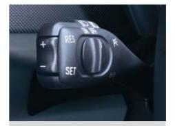
As of 30 kph **cruise control** keeps the speed at the level selected by you without you having to depress the accelerator. Cruise control is switched off again automatically as soon as the brakes or clutch are operated.
