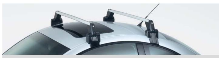
The **basic carrier** can be fitted quickly and easily to the New Beetle and is the basis for all roof attachments. The mechanism is of galvanised sheet steel with a theft-deterrent fastener. Net weight: approx. 6 kg. Max. roof load: 50 kg.
