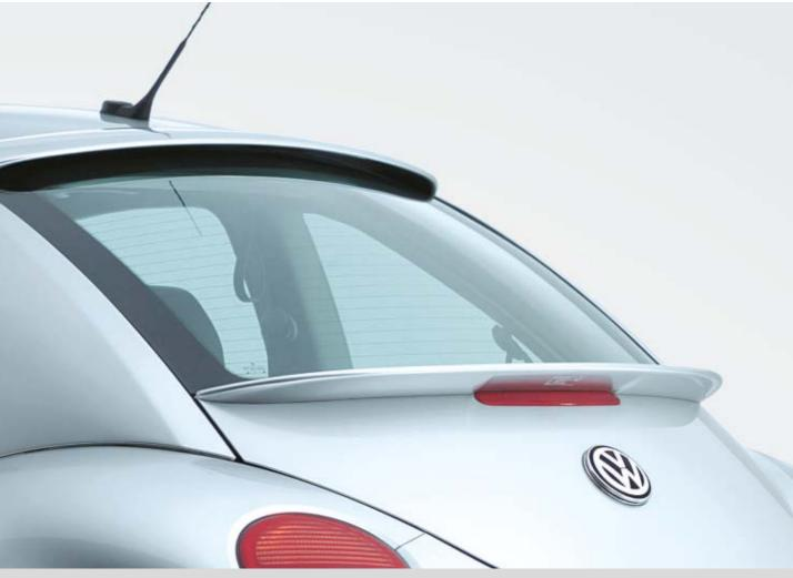
The **roof edge and tailgate spoiler** complement each other in an ideal way which above all results in aerodynamic advantages on the New Beetle – and adds a distinctly sporty look.
